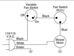
Figure 65 - Blower Wiring Diagram for Thermostat-Controlled Models
